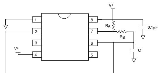
$$\begin{aligned} \text{Frequency } f &= 1.46 / (R_A + 2R_B)C \\ \text{Duty Cycle DC} &= R_B / (R_A + 2R_B) \end{aligned}$$
