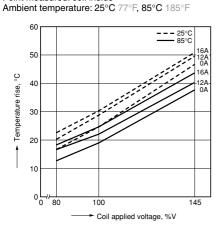
1.-(2) Coil temperature rise (200mW type) Sample: ALE74B12, 6 pcs.
