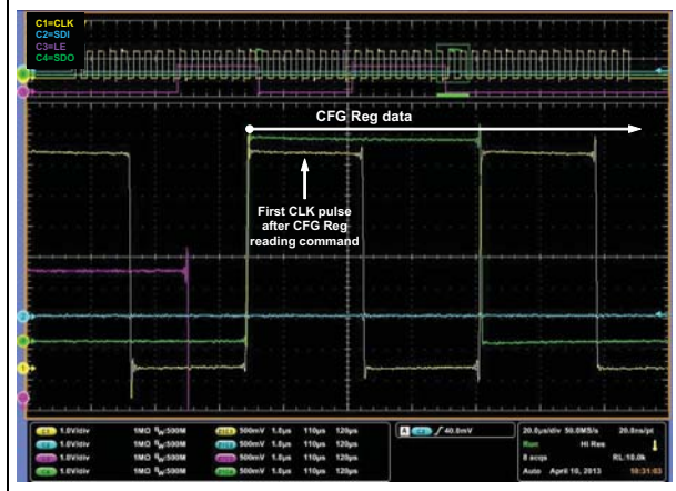
Figure 13. Configuration register reading sequence (zoom)
