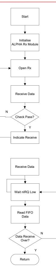
After Initialisation, open FIFO receive mode and wait for nIRQ low, only then can the MCU read received and stored data in FIFO. For the next received package please reset FIFO
