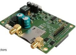
The ZOOM series of GPRS and 3G / UMTS socket modems are fully designed, developed and ready to integrate into your equipment, easily, and with a low overall cost.
