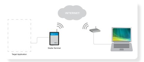
V-Link 232 has been designed to create an out-of-box usable wireless replacement to an RS232 / USB cable of any length.
