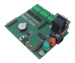
The ZOOM-EVK evaluation and development board is the perfect way of getting to know the ZOOM series of socket modems, and building an application for integration into your equipment. The ZOOM modem plugs directly onto the EVK providing convenient access to all of the ZOOM interfaces via the EVK's D-Sub, USB and terminal block connectors. This includes the TTL, RS232 and USB interfaces, allowing you to control the modem from a connected PC or embedded micro controller.
