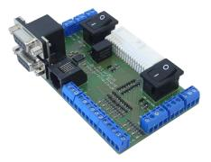
The ZULU/ZEUS-EVK evaluation and development board is the perfect way of working with the ZULU/ZEUS modems, and developing an application within the ARM Cortex processor. The EVK provides simple and convenient access to the ZULU/ZEUS interfaces through standard D-Sub and terminal block connectors.
