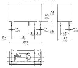
$\begin{array}{lll} \underline{\text{Dimension:}} & \underline{\text{Tolerance}} \\ \text{Less than 1mm .039inch:} & \pm 0.1 \pm .004 \\ \text{Min. 1mm .039inch less than 3mm .118 inch:} & \pm 0.2 \pm .008 \\ \text{Min. 3mm .118 inch:} & \pm 0.3 \pm .012 \\ \end{array}$
