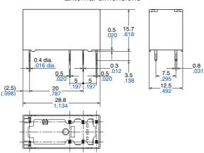
$\begin{array}{ll} \underline{\text{Dimension:}} & \underline{\text{Tolerance}} \\ \text{Less than 1mm .039inch:} & \pm 0.1 \pm .004 \\ \text{Min. 1mm .039inch less than 3mm .118 inch:} & \pm 0.2 \pm .008 \\ \text{Min. 3mm .118 inch:} & \pm 0.3 \pm .012 \\ \end{array}$
