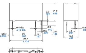
$\begin{array}{lll} \underline{\text{Dimension:}} & \underline{\text{Tolerance}} \\ \text{Less than 1mm .039inch:} & \pm 0.1 \pm .004 \\ \text{Min. 1mm .039inch less than 3mm .118 inch:} & \pm 0.2 \pm .008 \\ \text{Min. 3mm .118 inch:} & \pm 0.3 \pm .012 \\ \end{array}$
