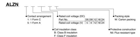
Notes: 1. The "W" at the end of the part No. only appears on the inner and outer packaging It does not appear on the relay itself.
