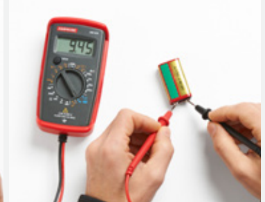
Check 1.5 V and 9 V batteries
