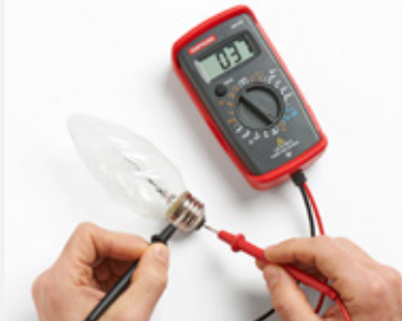
Troubleshoot light bulbs and fuses with the continuity function
