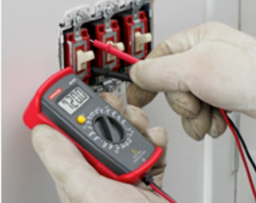
Accurately measure voltage up to 250 V in receptacles, switches, extension cords and light fixtures
