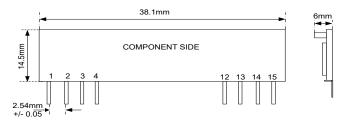
NOTES Pins on 0.1" pitch Pin Dims: 0.6 x 0.02mm Pin Length: 6mm +/-0.2 Recommended PCB hole: Ø 0.65 – 0.7mm
