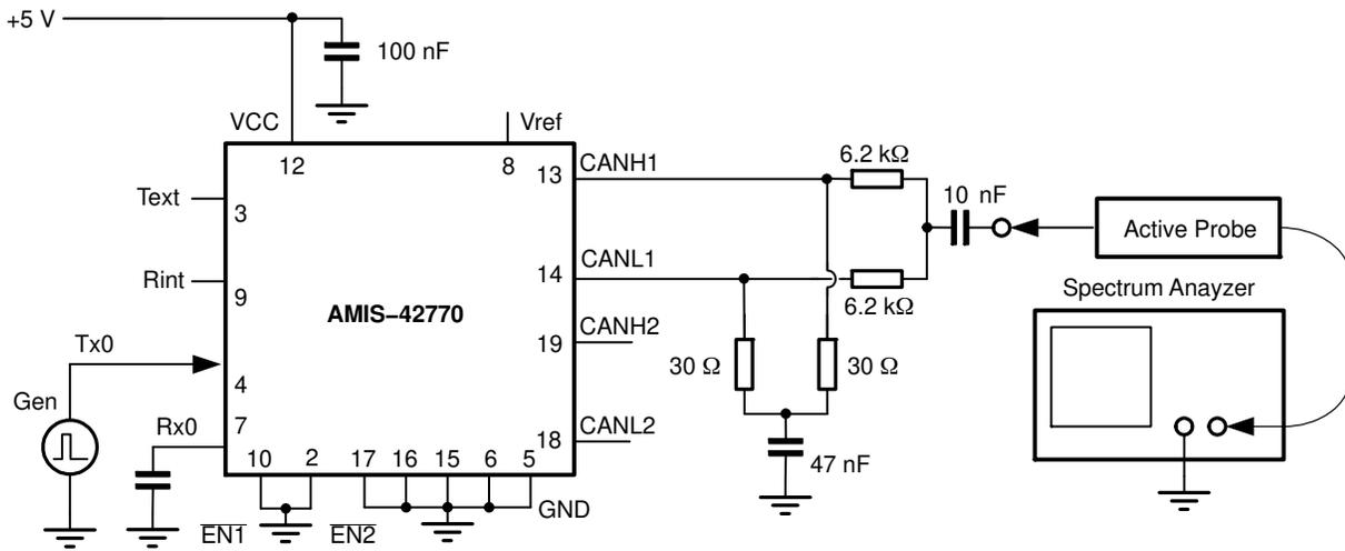
Figure 10. Basic Test Set-up for Electromagnetic Measurement
