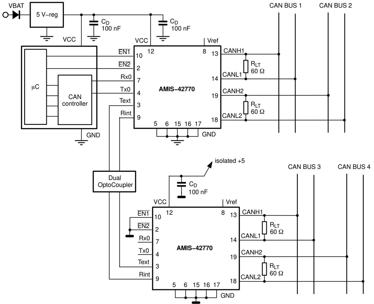
Figure 4. Application Diagram CAN-bus Extender
