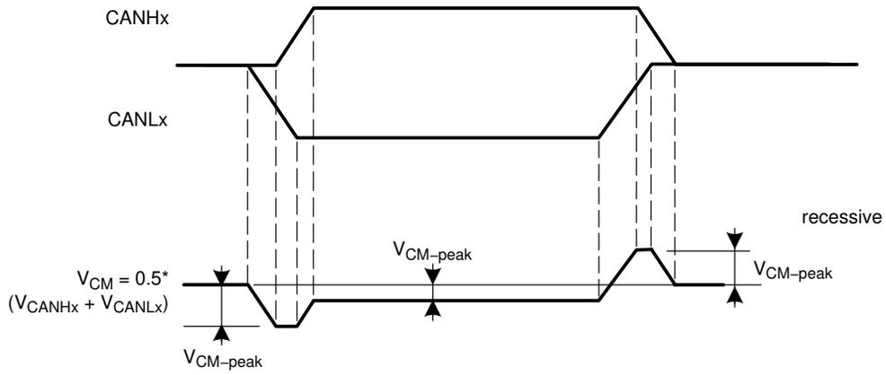
Figure 11. Common-mode Voltage Peaks (see Measurement Set-up Figure 10)
