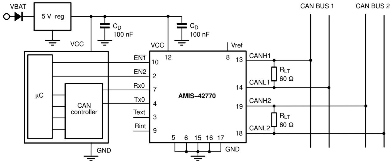
Figure 3. Application Diagram Dual-CAN
