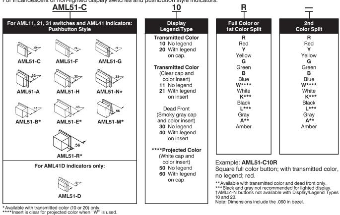
AML51 LENS ORDER GUIDE (All possible color combinations may not be available.) AML51 lens buttons provide added dis-For incandescent display AML41J, K, and L lens style indicators only.
