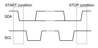
Every byte put on the SDA line must be 8-bits long. The number of bytes that can be transmitted per transfer is unrestricted. Each byte has to be followed by an acknowledge bit. Data is transferred with the most significant bit (MSB) first.
