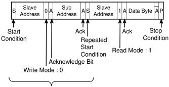
Sub-address should be assigned first.
