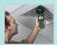
Extech's 4" (10cm) Large Vane Thermo-Anemometer series allows for more precise readings on larger size ducts. Each meter simultaneously displays Airflow or Air Velocity and Temperature. Choose models that also measure Air Volume, Humidity & Carbon Dioxide (CO<sub>2</sub>).
