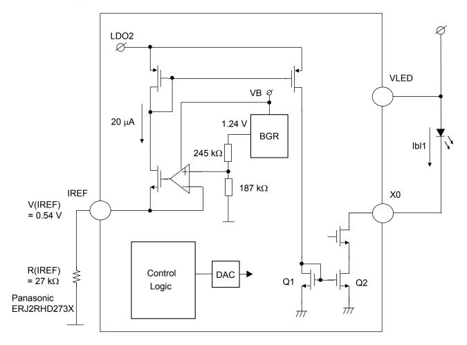
The constant current equivalent circuit example (X0 pin) for LED driver is shown in the above figure. The reference current for constant current driver is calculated by the following formula.
