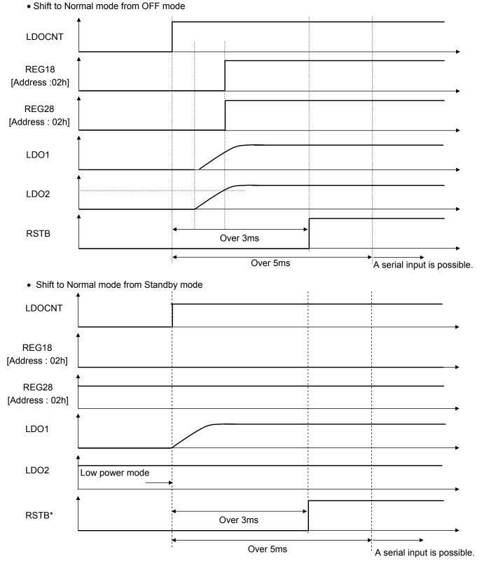
Note) The above waveform is under the condition that the register setup is reset in standby mode. Maintain the state of RSTB = High to hold the register setup.
