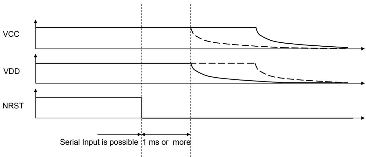
Note: For the Shut down Timing of VCC and VDD, it is possible to be changed.
