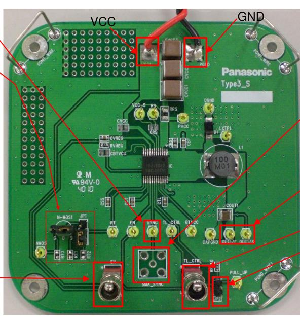
SMA\_SYNC (BNC terminal for external clock)
