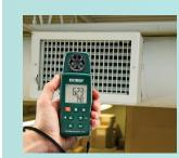
Convenient 4-in-1 Anemometer measures Air Velocity, Air Flow, Air Temperature, and Type K Temperature. Built-in low friction ball bearing mini vane wheel for high accuracy. The Type K temperature probe function measures surface temperature up to 2372°F (1300°). Features large dual LCD with backlighting, Data Hold, and Min/Max function.
