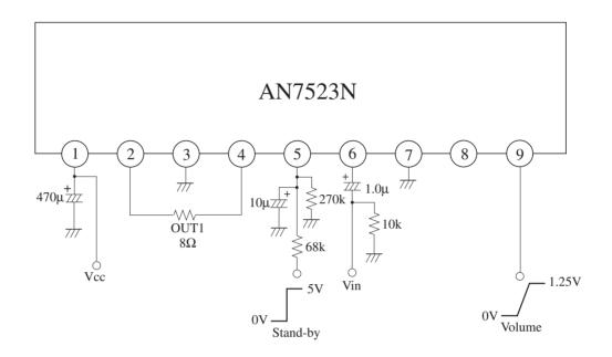
Note) If the standby pin is open or 0V, the IC is on standby state.
