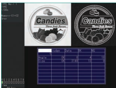
Simultaneous image display from two cameras (This shows an image processed with gray scale and binary differentiation.)
