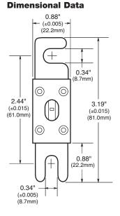
Catalog Symbol: ANN Very Fast-Acting Ampere Rating: 10 to 800A Voltage Rating: 125Vac (or less) 80Vdc (or less) Interrupting Rating: 2,500A ac,
