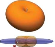
Gain is also related to the overall physical size of the antenna, as well as surrounding materials. As the geometry of the antenna is reduced below the effective wavelength (considered an electrically small antenna) the gain decreases. Also, the relative distance between an electrically small antenna and its associated ground impacts antenna gain.
