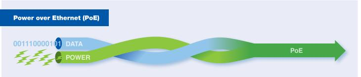
Power over Ethernet (PoE) is a method to transmit power and data, up to 100 meters, over a single Ethernet (CAT5e/CAT6/CAT6a) cable. The benefits of PoE include reduced wiring and installation costs and greater flexibility of device placement as equipment no longer needs to be located near power outlets. Red Lion offers a wide range of PoE products including Ethernet switches, midspan injectors and PoE splitters, that support industry-standard IEEE 802.3af (PoE) and/or IEEE 802.3at (PoE+).
