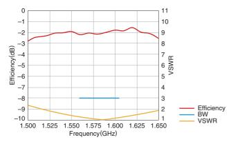
• Tested antenna has been soldered. Evaluation board size is 80x10x1 mm.
