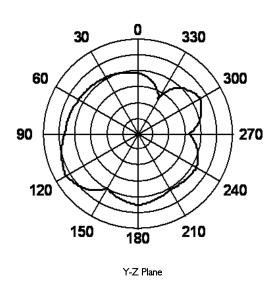
Fig. 4 Antenna radiation patterns at 2.45 GHz
