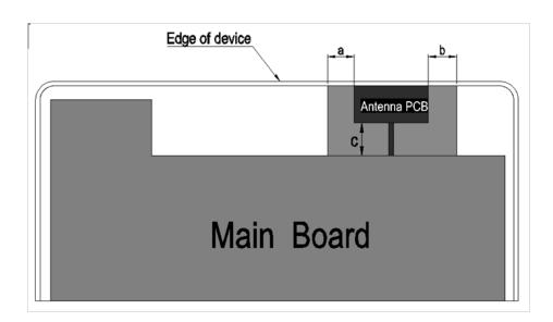
Antenna element should be placed at the edge of device, has minimum clearance from metalic object:
