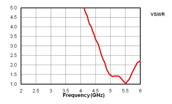
Fig. 3 Return loss & VSWR Measurement
