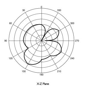
**Fig. 5** Antenna radiation patterns at 5.350 GHz
