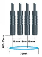
When high-intensity heads equipped with ANUJ6475S (cylindrical lens) are used with 18 mm pitches as shown in the figure, an entire linear area of approx. 70 mm wide can be reliably irradiated at 350 mW/cm² or higher intensity.
