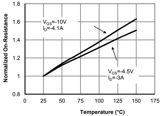
**Figure 4: On-Resistance vs. Junction Temperature (Note E)**
