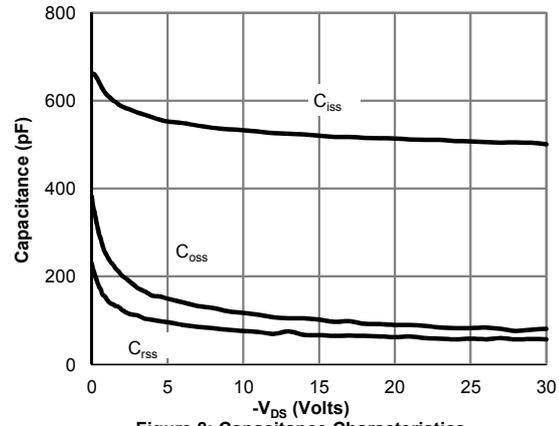
**Figure 8: Capacitance Characteristics**
