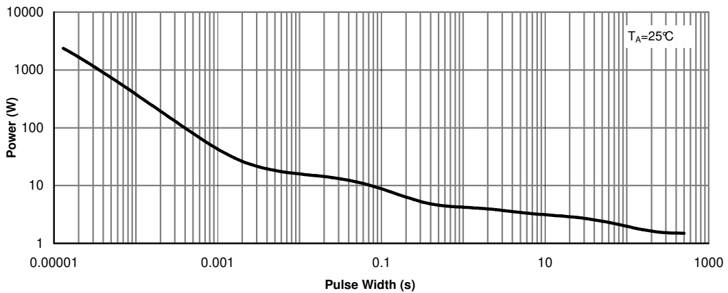
Figure 11: Single Pulse Power Rating Junction-to-Ambient (Note F)
