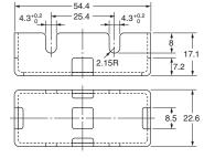
Note: The Cover has five holes for easy lead wire connections.
