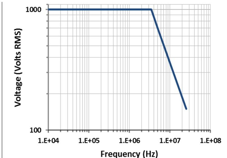
**NOTE:** The voltage vs frequency derating curve provides the maximum voltage that can be applied to the probe inputs without risking damage to the probe or injury to the user from possible burns at higher frequencies.
