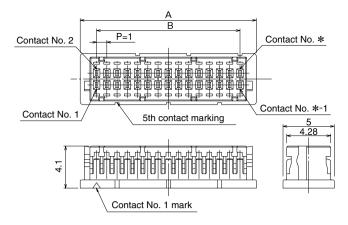
Shown with terminated and installed contacts
