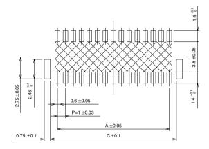
Note : Shaded area must be free of any electrically conductive traces to avoid contact with soldered pin header terminations.
