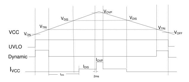
Figure 1. Typical Waveforms of AP4341S
