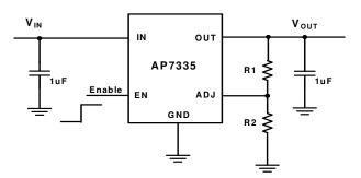
The output voltage is calculated by:
