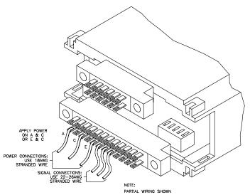
An optional 24-pin (Model ACE1) for 3 and 4 digit slaves and 24 & 12-pin (Model ACE4) for 5 and 6 digit slaves, provide another way to make connection. These edgecard connectors have 0.156" center to center spacing and require the soldering of the wires to the connector for wire termination. The diagram above shows edgecard connectors being used with the Slave Display.
