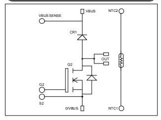
$$\begin{split} V_{DSS} &= 600 V \\ R_{DSon} &= 18 m \Omega \ max \ @ \ Tj = 25 ^{\circ} C \\ I_D &= 143 A \ @ \ Tc = 25 ^{\circ} C \end{split}$$
