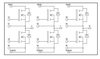
$$\begin{split} V_{DSS} &= 600V \\ R_{DSon} &= 35 m\Omega \text{ max } @ \text{ Tj} = 25^{\circ}\text{C} \\ I_D &= 72 \text{A} @ \text{ Tc} = 25^{\circ}\text{C} \end{split}$$
