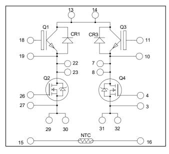
Top switches : Trench + Field Stop IGBT3 Bottom switches : Super junction MOSFET
