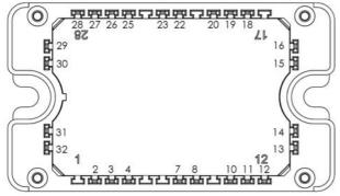
All multiple inputs and outputs must be shorted together 13/14 ; 22/23 ; 29/30 ; 31/32
