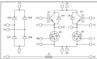
Top switches: Trench + Field Stop IGBT3
