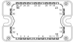
Pins 29/30/31/32 must be shorted together Pins 26/27/28/22/23/25 must be shorted together to achieve a phase leg Pins 16/18/19/20 must be shorted together
