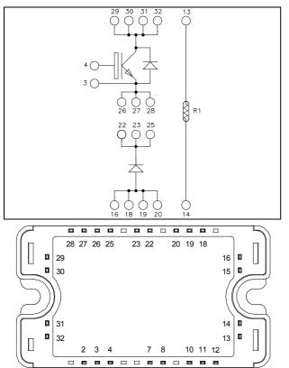
Pins 29/30/31/32 must be shorted together Pins 26/27/28/22/23/25 must be shorted together to achieve a phase leg Pins 16/18/19/20 must be shorted together
