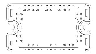
$V_{CES} = 1200V$  $I_{C} = 25A$  @  $T_{C} = 80^{\circ}C$
