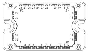
Pins 20, 24 & 26 must be shorted together to perform a 3 phase bridge.
