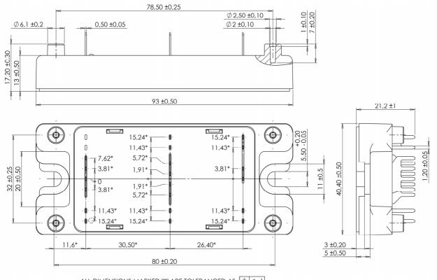
ALL DIMENSIONS MARKED "\*" ARE TOLERANCED AS : [ 🌵 Ø 1
