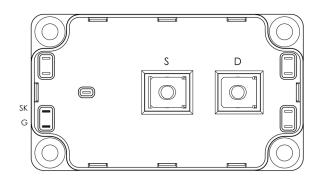
$$\begin{split} V_{DSS} &= 1200 V \\ R_{DSon} &= 100 m \Omega \text{ typ } \text{ } \text{ } \text{ } \text{Tj} = 25^{\circ} \text{C} \\ I_D &= 116 A \text{ } \text{ } \text{ } \text{0} \text{ } \text{Tc} = 25^{\circ} \text{C} \end{split}$$
