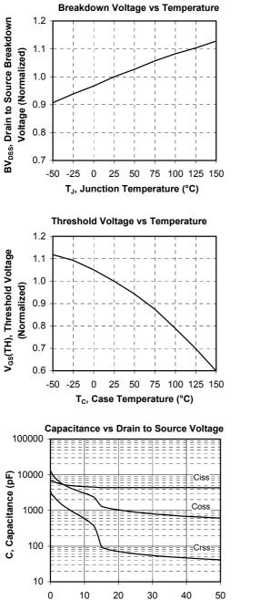
V<sub>DS</sub>, Drain to Source Voltage (V)
