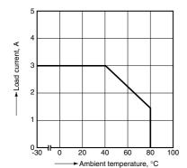
1.-(2) Load current vs. ambient temperature (AC output, 10 A type) Part No.: AQ10A2-ZT4/32VDC (A) When not using a heat sink
