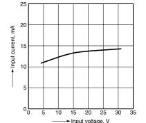
3.-(2) Input current vs. input voltage characteristics
