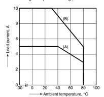
1.-(3) Load current vs. ambient temperature (DC output, 1 A and 2 A types) Part No.: AQ1AD2-3/ 28VDC and AQ2AD1-3/28VDC
