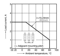
4.-(2) Load current vs. ambient temperature characteristics for adjacent mounting (AC output, 10A type)
