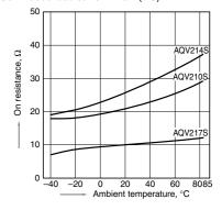
2.-(3) On resistance vs. ambient temperature characteristics
