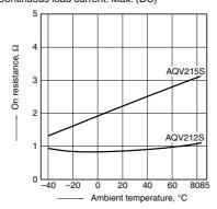
2.-(2) On resistance vs. ambient temperature characteristics
