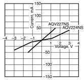
9. Off state leakage current
