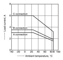
1.-(2) Load current vs. ambient temperature characteristics
